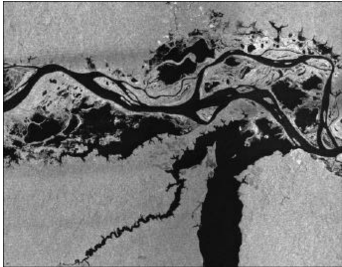
RADARSAT provides excellent land/water delineation, as this image clearly shows. The forests adjacent to Lago Grande, Brazil experience seasonal flooding, and the dark areas on this image represent the high water mark and flooded areas, while the forested areas are of a lighter tone.
